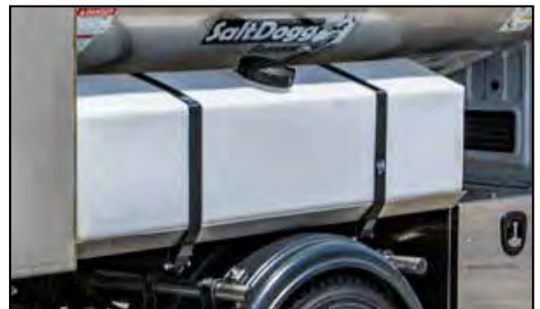
Integrated pre-wet system with LS15 (twin 80 gallon tanks)
