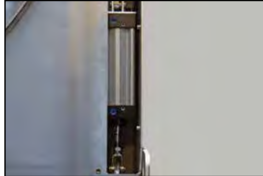
Dual air tailgate cylinders standard
