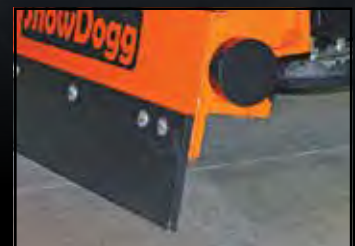
3-1/2" x 3-1/2" x 1/2" cutting edge angle and 3-1/2" x 2-1/2" x 1/2" rear angle with edge guard
