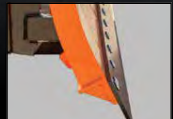
Reinforced 3-1/2" x 3-1/2" x 1/2" bottom angle
