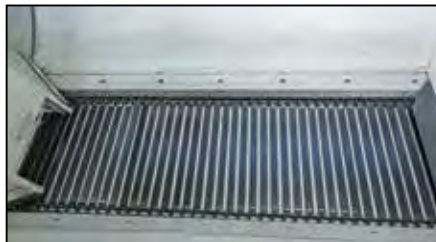
30.25" wide conveyor with 1/2" bars and dual 6:1 gearbox drive
